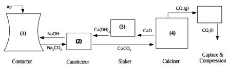
Figure B.1. Top level process diagram of an example direct air capture system. Closed chemical loops of NaOH and CaO extract CO<sub>2</sub> from air convert it to a pure, compressed form for sequestration.
